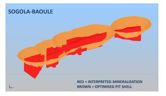
Mineralisation captured within conceptual open pits totals 14Mt at 1.2%  $\rm Li_2O$ , with mineralisation remaining open along strike and beneath the conceptual open pits
