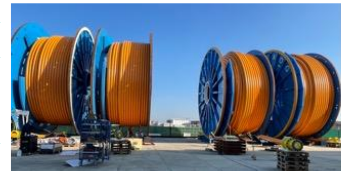
Strohm's TCP ready for installation offshore
