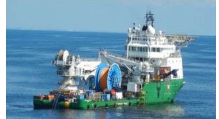
Strohm's low carbon footprint pipeline's installation offshore
