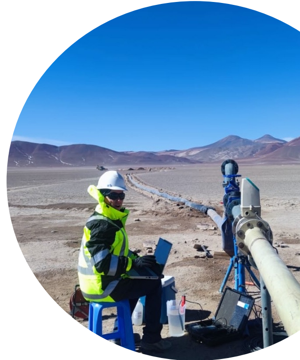
Preliminary pump test at Francisco Basin, May 2023
