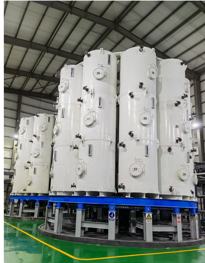
Lanshen's demonstration plant for extracting lithium from brine Source: Lanshen New Material Technology Co.Ltd.
